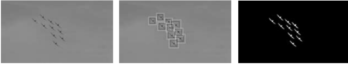
Fig. 8: Objects detected robustly over dynamic background (clouds, vapour trails, lighting).
