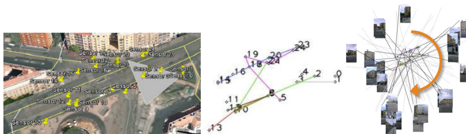
Fig. 6: Location of sensors (cameras, images) (left); built and clustered vision graph structure (middle); same graph structure also showing the orientation and location of the images (right).
