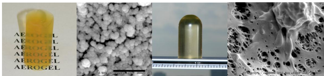
Figure 1 Functionalized aerogel sample, its SEM structure and the monolith recovered after embedding in PMMA. Leaching out of silica from the matrix after SBF treatment, leaving pores behind.
