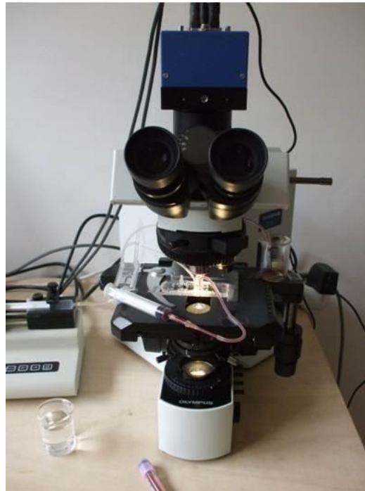
Figure 10. Prototype system for microfluidic flow cytometric applications. Main parts: syringe pump, upright biological microscope, hydrodynamic focusing microfluidic channel system, high-fps camera computer for real-time imaging.
