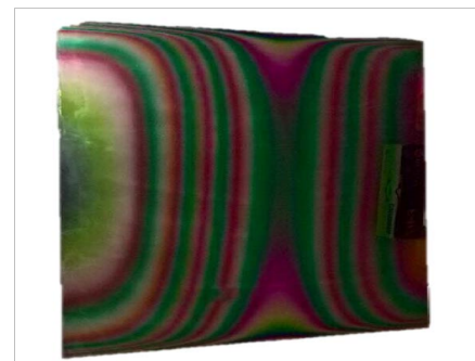
Fig. 5 Schematic picture of the deposition arrangement and the photograph of 30x30cm substrate with composition-gradient layers. Newtonian rings show thickness gradient
