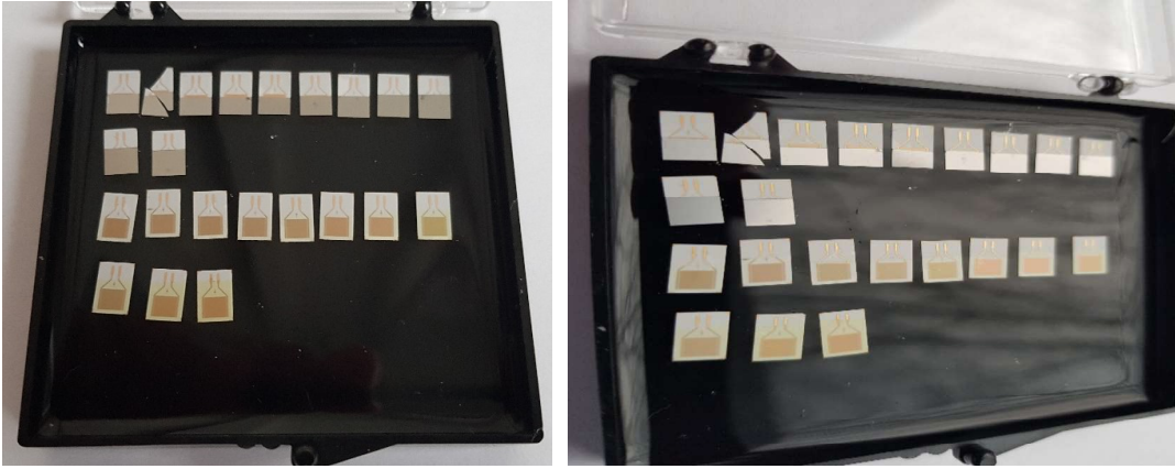
Fig. 9 Photographs (from different view-angle) of W\text{O}_3/\text{MoO}_3 (lower) or W\text{O}_{3-x}/\text{MoO}_{3-x} (upper) combinatorial sets on heat-able sensor chips. Left hand side is W-rich, right one is Mo-rich. No. 6 (middle one) is expected to be 50-50% in both cases. The upper rows show suboxides (semi-transparent layers, No. 2 was broken during tweezer handling) The bottom rows show oxides (transparent layers)
