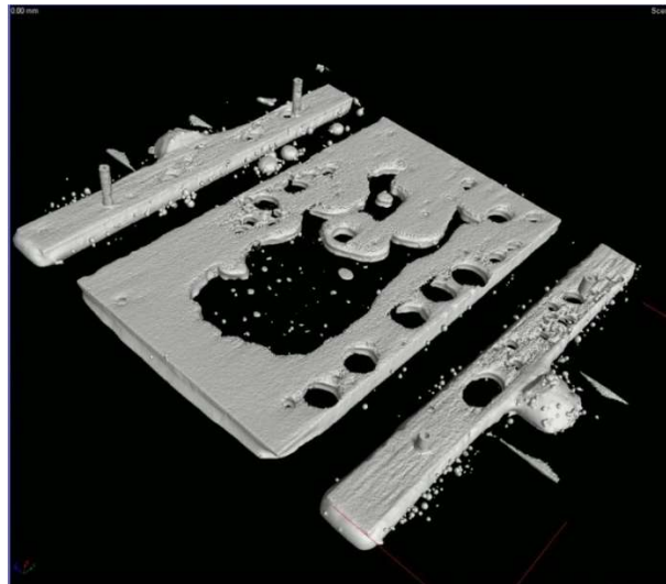
Fig. 9. Three-dimensional (3D) CT image of a SACX0307-ZnO-(50 nm) solder joint [19].
