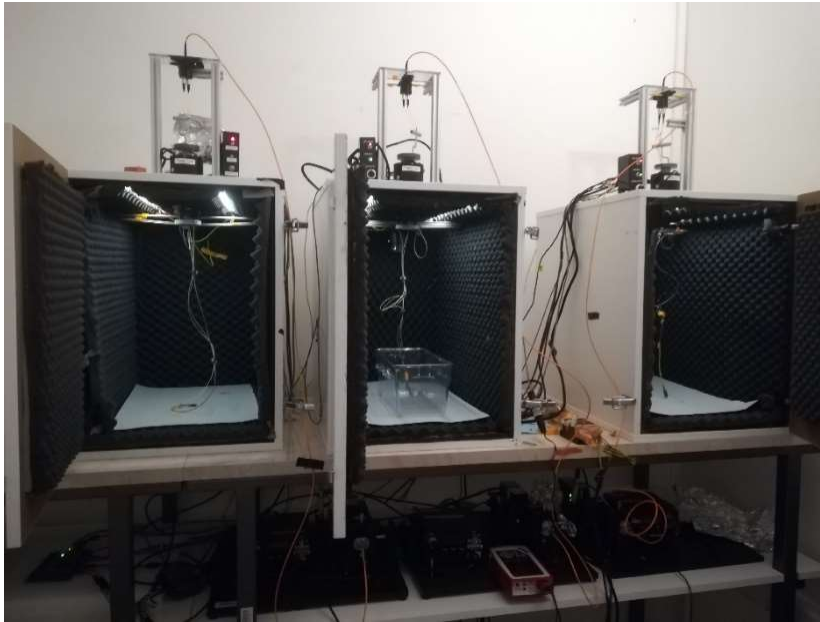
Figure 1. Identical behavioral boxes to study the mechanisms of stress induced sleep disturbances in parallel experiments. Commutators are visible on the top of the boxes, laser apparatus for optogenetic manipulations are placed below the boxes. The box contains sound insulation, adjustable led illumination and digital cameras.
