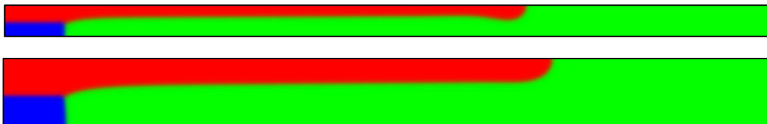
Figure 13: Phase-field simulation of the non-coupled melting of a lamellar structure of different widths [7]. The initial ratio of the red and blue phases is 0.55:0.45, and only one half of a lamella is shown. The temperature increases from left to right while reference frame travels from right to left, providing stationary profiles within the simulation domain that corresponds to steady state melting. The red phase becomes the “leading phase” extending deep into the melt.
