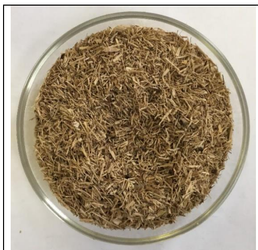
Fig. 2 Bagasse fiber used for the reinforcement of PP
