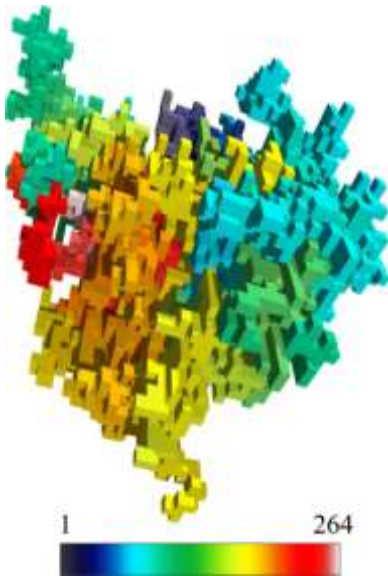
Figure 1: An avalanche of breaking fibers in three dimensions. The color code indicates the time evolution of spreading.
