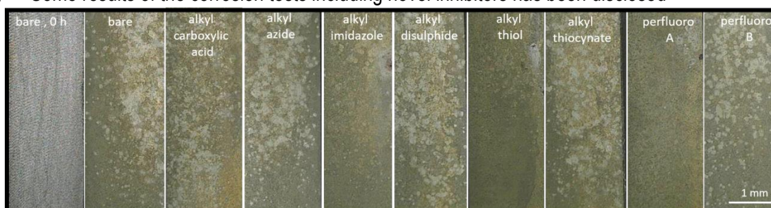
Figure 1: Images of bare AlSi9Cu3 aluminium alloy before immersion, bare alloy after immersion, and alloys coated with different types of inhibitor coatings after immersion for 7 days in 0.6 M NaCl.
