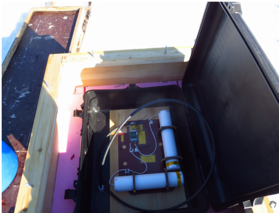
Figure 1. The search coils and line driver on the assembly board inside the waterproof HPRC box placed into the insulated wooden box.
