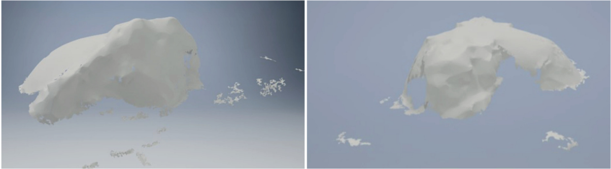
Figure 3.16: 3D images of the capitulum bone a) (left) before the compressive test (intact) b) (right) after the compressive test (failed)
