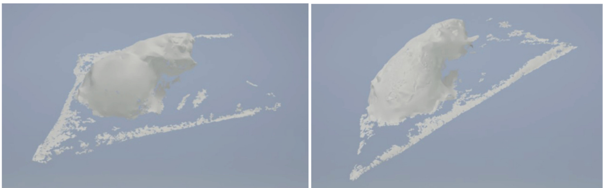
Figure 3.18: 3D images of the scaphoid bone a) (left) before the compressive test (intact) b) (right) after the compressive test (failed)
