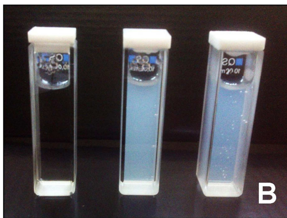
Figure 4. The extent of transmittance recovery ( Y_H ) as a function of TMSPMA content in the P(NIPAAm-co-TMSPMA) copolymers (A) and photographs of the copolymer (sample co_1) solutions before the first heating, and after the first and second cooling cycles (left to right) (B) (conditions: 0.1 wt% P(NIPAAm-co-TMSPMA), 0.2 °C/min heating rate with 5 min equilibration, 488 nm).
