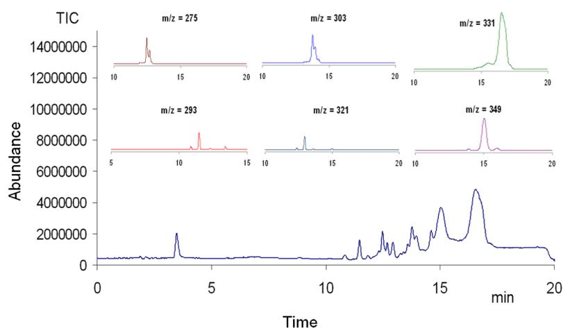
*Figure 1.* LC-MS chromatogram (total ion count, TIC) recorded by applying high buffer concentration (100 mM) and extracted ion chromatograms (*inserts*). The total ion chromatogram indicates a complex composition of alkanesulfonic acid derivative surfactants, with individual components of molecule ions ( $m/z$ ) of 275, 293, 303, 321, 331 and 349 shown in the inserts.
