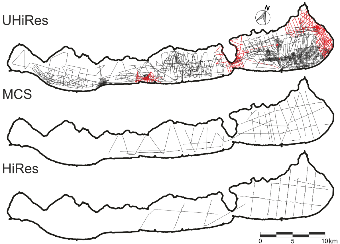
Figure 2. Maps showing high to ultrahigh resolution seismic profiles at Lake Balaton. Black lines indicate 2D lines that were available in 2012 at the beginning of the projects, red lines indicate profiles that have been recorded during the project period, between 2013 and 2018.
