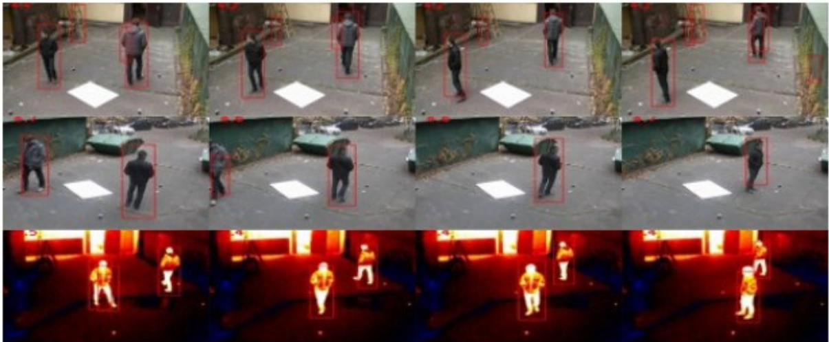
Frames of three different cameras and the detection results (the third camera was an infra one).
