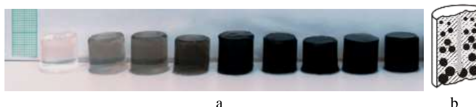
Figure 8 PNIPA hybrid gel cylinders with increasing CNT content (a) and the internal surface as used for SEM sample preparation (b)
