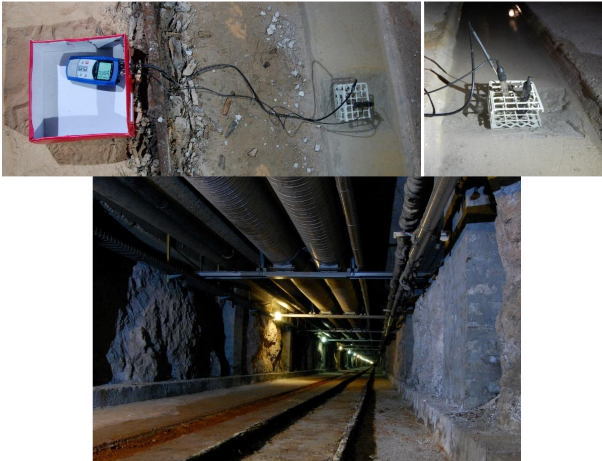
Fig. 9. a) The measuring devices in the inflow and outflow locations of the canal. b) The Gellért Tunnel with the canal (photos: Hegedűs A. and Csondor K.) (Bodor and Mádl-Szőnyi 2017b)
